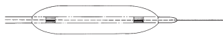
Fig. 7.35 A dilating balloon placed over a guidewire; the radio-opaque metal markers show up.
